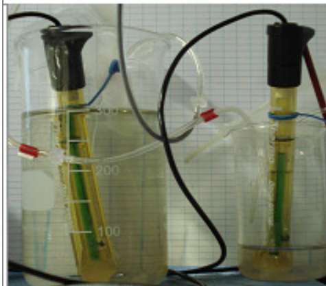
Figure 3. Graph presents the water flow during the experiment from cathode to anode, while the picture on the right shows the difference in water level after 12 days of experimental time
